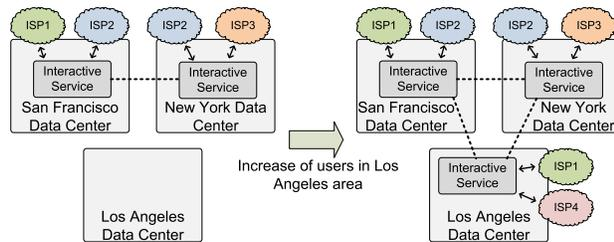
**Figure 4: Flexible peering and hosting for interactive applications:** Direct control over routing allows services to expand hosting and upstream connectivity in response to changing demands. In this example, a service experiences an increase in users in a single geographic area. In response, it adds hosting and peering at that location to allow customers at that location to easily reach the service.
