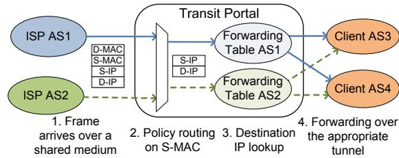
**Figure 5: Forwarding incoming traffic:** When a packet arrives at the Transit Portal (Step 1), the TP uses the source MAC address (S-MAC) to demultiplex the packet to the appropriate IP forwarding table (Step 2). The lookup in that table (Step 3) determines the appropriate tunnel to the client network (Step 4).
