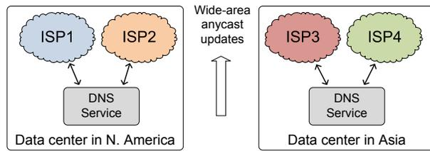
Figure 2: *Reliable, low-latency distributed services:* A service provider that hosts authoritative DNS for some domain may wish to provision both hosting and anycast connectivity in locations that are close to the clients for that domain.
