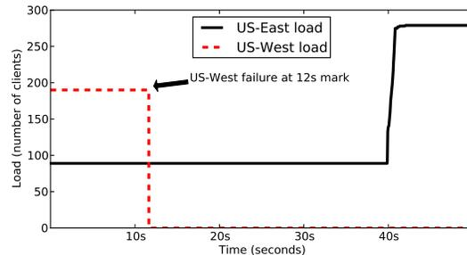
Figure 10: Failover behavior with two IP anycast servers.
