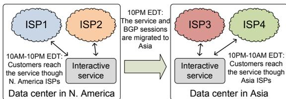
**Figure 3: Using routing to migrate services:** A service provider migrates a service from a data center in North America to one in Asia, to cope with fluctuations in demand. Today, service providers must use DNS for such migration, which can hurt user performance and does not permit the migration of a running service. A provider can use route control to migrate a service and re-route traffic on the fly, taking DNS out of the loop and enable migration of running services.
